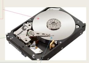
Read/write heads, one per platter side. Float extremely close to the platters and detect or modify magnetic domains as the spinning disk brings them under the heads.
