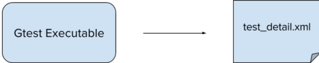
Figure 5: The current version of AutoGrader (V2.0) compiled and ran a single gtest (C++) executable once, resulting in one XML report document. The single gtest execution is responsible for the single runtime and timeout error bar generated with the current version of AutoGrader.
