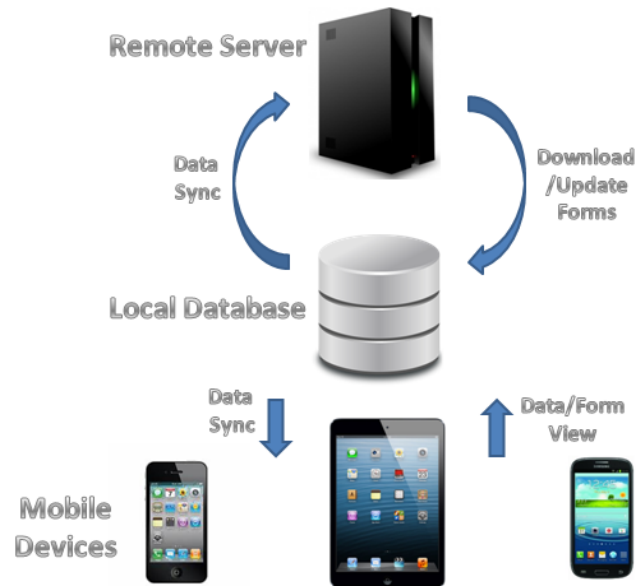
Figure 1: High-end overview of TalKivi Mobile Client
