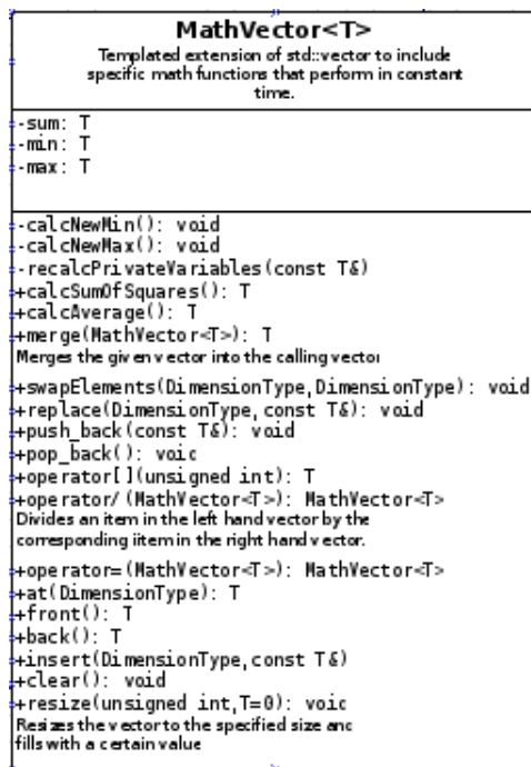
FIGURE 2 - UML OF THE MATHVECTOR DATA STRUCTURE
